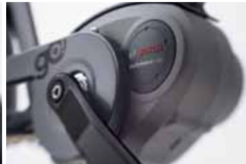
BOSCH PERFORMANCE ELECTRIC ASSIST SYSTEM WITH 250W MID-FRAME MOTOR
